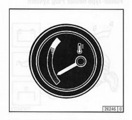
The pointer of the temperature indicator should remain in the green sector and enter the yellowgreeen sector only in exceptional cases. If the pointer enters the orange sector, the engine is overheating. Turn it off and establish the cause from the Diagnosis Chart (see 7.1).
